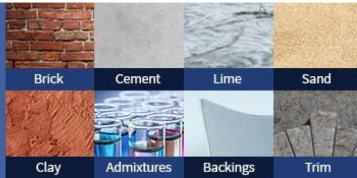
**Brick:** Since it is a porous material, brick may absorb soluble salts. To find out whether efflorescence will be a problem for your brick, take a single brick and immerse it in distilled water for approximately seven days. Let the brick dry after the seven days and compare it to a brick that was not immersed. If you notice a white, powdery material on the brick, it likely has effloresced.
